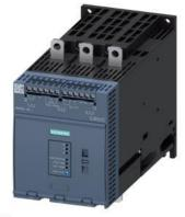
SIRIUS soft starter 200-600 V 171 A, 24 V AC/DC Screw terminals Analog output
