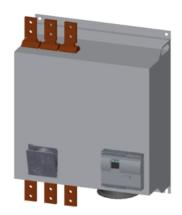
SIRIUS soft starter Values at 460 V, 50 °C standard: 1076 A, 950 hp Inside-delta: 1864 A, 1700 hp 200-460 V AC, 115 V AC spring-type terminals !!! Phased-out product !!! Successor is SIRIUS 3RW5, Preferred successor type is >>3RW5558-2HA14<<
