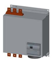
SIRIUS soft starter Values at 400 V, 40 °C standard: 551 A, 315 kW Inside-delta: 954 A, 560 kW 200-460 V AC, 230 V AC Screw terminals !!! Phased-out product !!! Successor is SIRIUS 3RW5, Preferred successor type is >>3RW5548-6HA14<<
