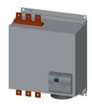
SIRIUS soft starter Values at 575 V, 50 °C standard: 494 A, 500 hp Inside-delta: 856 A, 950 hp 400-600 V AC, 115 V AC Screw terminals !!! Phased-out product !!! Successor is SIRIUS 3RW5, Preferred successor type is >>3RW5548-6HA16<<
