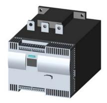
SIRIUS soft starter Values at 690 V, 40 °C standard: 432 A, 400 kW Inside-delta: only up to 600 V 400-690 V AC, 230 V AC Screw terminals !!! Phased-out product !!! Successor is SIRIUS 3RW5, Preferred successor type is >>3RW5547-6HA16<<
