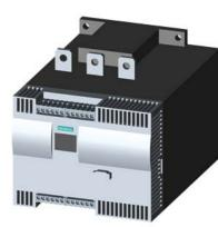
SIRIUS soft starter Values at 460 V, 50 °C standard: 315 A, 250 hp Inside-delta: 546 A, 450 hp 200-460 V AC, 115 V AC Screw terminals !!! Phased-out product !!! Successor is SIRIUS 3RW5, Preferred successor type is >>3RW5546-6HA14<<
