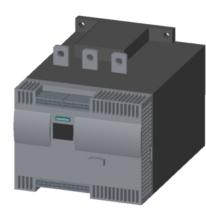
SIRIUS soft starter Values at 500 V, 40 °C standard: 356 A, 250 kW Inside-delta: 617 A, 450 kW 400-600 V AC, 230 V AC spring-type terminals !!! Phased-out product !!! Successor is SIRIUS 3RW5, Preferred successor type is >>3RW5546-2HA16<<
