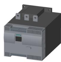
SIRIUS soft starter Values at 500 V, 40 °C standard: 313 A, 200 kW Inside-delta: 542 A, 355 kW 400-600 V AC, 230 V AC spring-type terminals !!! Phased-out product !!! Successor is SIRIUS 3RW5, Preferred successor type is >>3RW5545-2HA16<<
