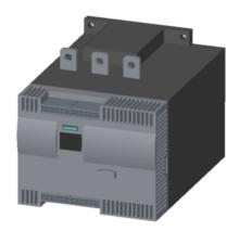
SIRIUS soft starter Values at 400 V, 40 °C standard: 313 A, 160 kW Inside-delta: 542 A, 315 kW 200-460 V AC, 230 V AC spring-type terminals !!! Phased-out product !!! Successor is SIRIUS 3RW5, Preferred successor type is >>3RW5545-2HA14<<
