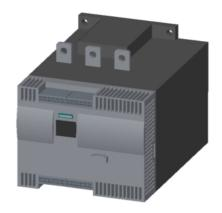
SIRIUS soft starter Values at 575 V, 50 °C standard: 280 A, 250 hp Inside-delta: 485 A, 500 hp 400-600 V AC, 115 V AC spring-type terminals !!! Phased-out product !!! Successor is SIRIUS 3RW5, Preferred successor type is >>3RW5545-2HA16<<
