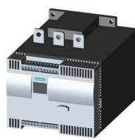
SIRIUS soft starter Values at 575 V, 50 °C standard: 215 A, 200 hp Inside-delta: 372 A, 350 hp 400-600 V AC, 115 V AC Screw terminals !!! Phased-out product !!! Successor is SIRIUS 3RW5, Preferred successor type is >>3RW5544-6HA16<<
