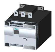
SIRIUS soft starter Values at 460 V, 50 °C standard: 215 A, 150 hp Inside-delta: 372 A, 300 hp 200-460 V AC, 115 V AC Screw terminals !!! Phased-out product !!! Successor is SIRIUS 3RW5, Preferred successor type is >>3RW5544-6HA14<<
