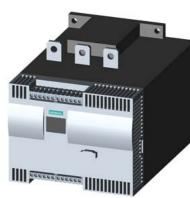
SIRIUS soft starter Values at 690 V, 40 °C standard: 203 A, 200 kW Inside-delta: only up to 600 V 400-690 V AC, 230 V AC Screw terminals !!! Phased-out product !!! Successor is SIRIUS 3RW5, Preferred successor type is >>3RW5543-6HA16<<
