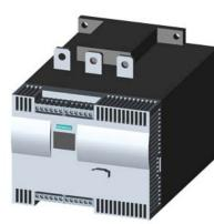
SIRIUS soft starter Values at 575 V, 50 °C standard: 180 A, 150 hp Inside-delta: 312 A, 300 hp 400-690 V AC, 115 V AC Screw terminals !!! Phased-out product !!! Successor is SIRIUS 3RW5, Preferred successor type is >>3RW5543-6HA16<<
