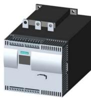
SIRIUS soft starter Values at 500 V, 40 °C standard: 162 A, 110 kW Inside-delta: 281 A, 200 kW 400-600 V AC, 230 V AC Screw terminals !!! Phased-out product !!! Successor is SIRIUS 3RW5, Preferred successor type is >>3RW5536-6HA16<<
