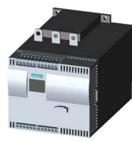
SIRIUS soft starter Values at 575 V, 50 °C standard: 145 A, 125 hp Inside-delta: 251 A, 250 hp 400-600 V AC, 115 V AC spring-type terminals !!! Phased-out product !!! Successor is SIRIUS 3RW5, Preferred successor type is >>3RW5536-2HA16<<
