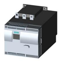
SIRIUS soft starter Values at 460 V, 50 °C standard: 145 A, 100 hp Inside-delta: 251 A, 200 hp 200-460 V AC, 115 V AC spring-type terminals !!! Phased-out product !!! Successor is SIRIUS 3RW5, Preferred successor type is >>3RW5536-2HA14<<
