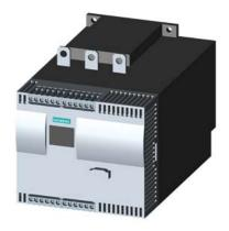
SIRIUS soft starter Values at 690 V, 40 °C standard: 134 A, 132 kW Inside-delta: only up to 600 V 400-690 V AC, 230 V AC spring-type terminals !!! Phased-out product !!! Successor is SIRIUS 3RW5, Preferred successor type is >>3RW5535-2HA16<<
