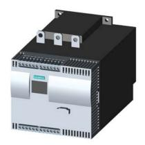
SIRIUS soft starter Values at 500 V, 40 °C standard: 134 A, 90 kW Inside-delta: 232 A, 160 kW 400-600 V AC, 230 V AC spring-type terminals !!! Phased-out product !!! Successor is SIRIUS 3RW5, Preferred successor type is >>3RW5535-2HA16<<
