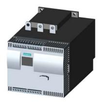
SIRIUS soft starter Values at 400 V, 40 °C standard: 134 A, 75 kW Inside-delta: 232 A, 132 kW 200-460 V AC, 230 V AC spring-type terminals !!! Phased-out product !!! Successor is SIRIUS 3RW5, Preferred successor type is >>3RW5535-2HA14<<
