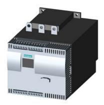
SIRIUS soft starter Values at 460 V, 50 °C standard: 117 A, 75 hp Inside-delta: 203 A, 150 hp 200-460 V AC, 115 V AC spring-type terminals !!! Phased-out product !!! Successor is SIRIUS 3RW5, Preferred successor type is >>3RW5535-2HA14<<
