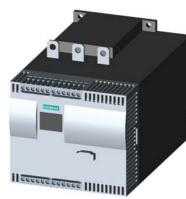
SIRIUS soft starter Values at 400 V, 40 °C standard: 113 A, 55 kW Inside-delta: 196 A, 110 kW 200-460 V AC, 230 V AC Screw terminals !!! Phased-out product !!! Successor is SIRIUS 3RW5, Preferred successor type is >>3RW5534-6HA14<<
