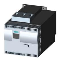
SIRIUS soft starter Values at 575 V, 50 °C standard: 32 A, 25 hp Inside-delta: 55 A, 50 hp 400-690 V AC, 115 V AC spring-type terminals !!! Phased-out product !!! Successor is SIRIUS 3RW5, Preferred successor type is >>3RW5524-3HA16<<
