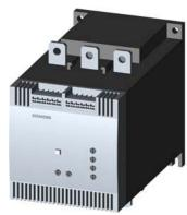
SIRIUS soft starter S12 356 A, 200 kW/400 V, 40 °C 200-460 V AC, 230 V AC spring-type terminals !!! Phased-out product !!! Successor is SIRIUS 3RW5, Preferred successor type is >>3RW5075-2AB14<<
