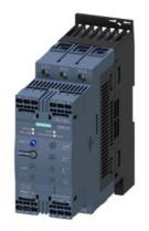
SIRIUS soft starter S2 45 A, 22 kW/400 V, 40  $^{\circ}\text{C}$  200-480 V AC, 24 V AC/DC spring-type terminals Thermistor motor protection
