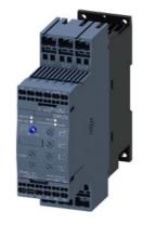
SIRIUS soft starter S0 38 A, 18.5 kW/400 V, 40  $^{\circ}$ C 200-480 V AC, 24 V AC/DC spring-type terminals Thermistor motor protection
